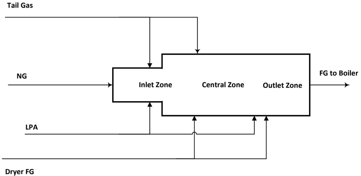
Fig.3 Illustration of new TOX concept with inlet, central and outlet zones
