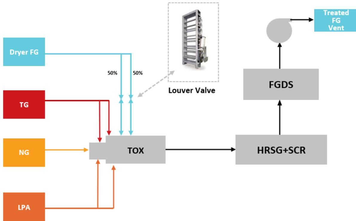
Figure 2. Block flow diagram for the new TOX design
