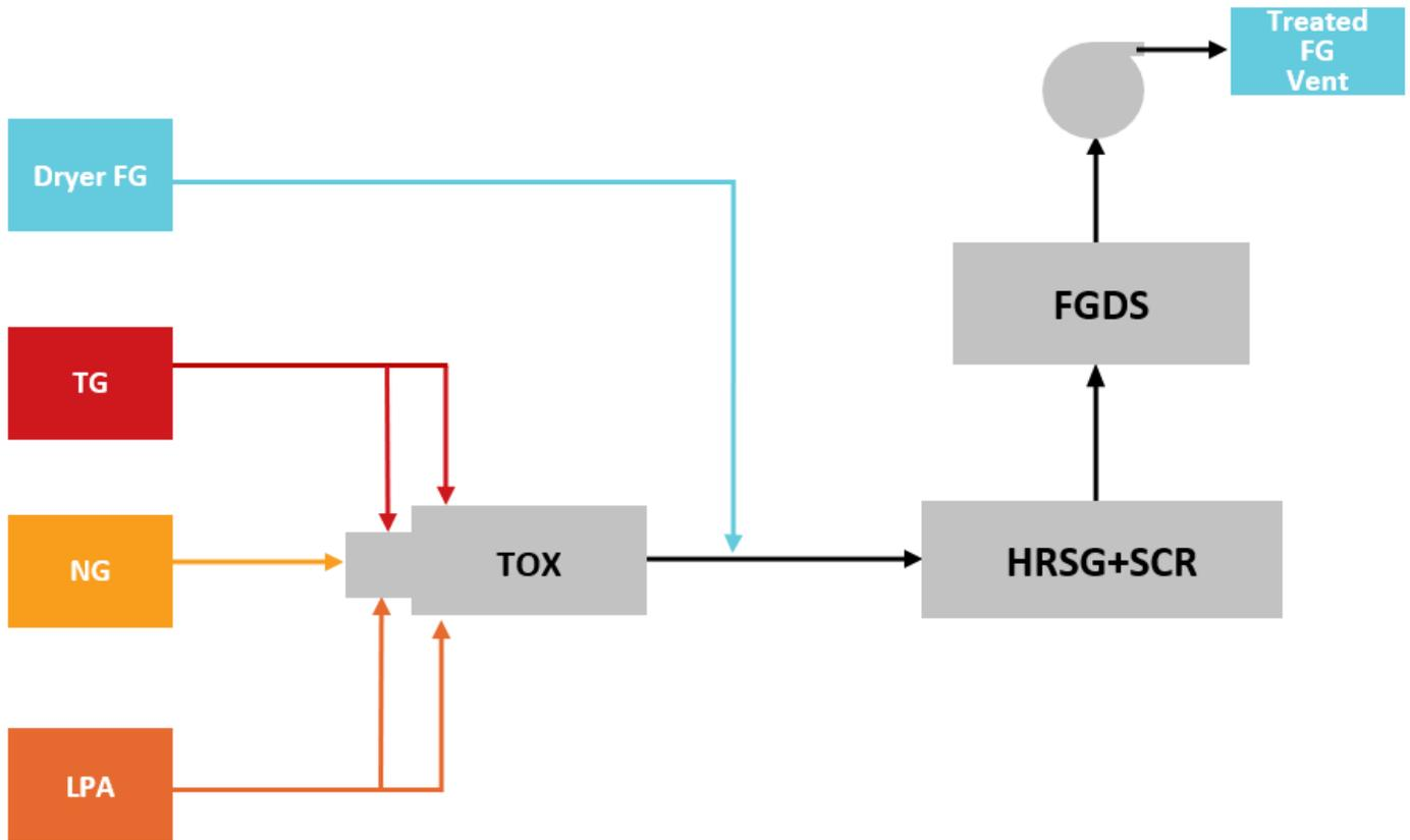
Figure 1. Conventional TG incinerator design block flow diagram
