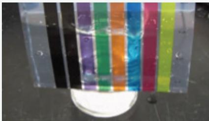
Demonstration of color fastness in water on nonporous substrate with CAB-O-SPERSE dispersions in substrate coating
