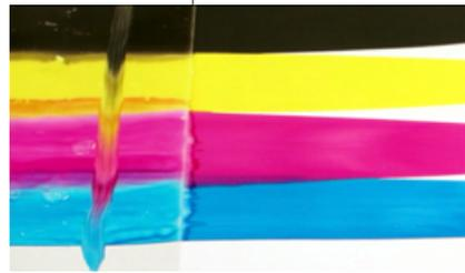
With CAB-O-SPERSE silica dispersion in the coating formulation, the coating and ink dries in seconds. Without the addition of CAB-O-SPERSE dispersion, drying takes hours (and hours).
