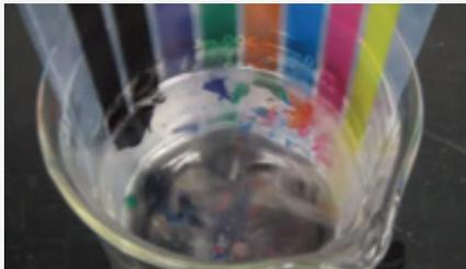
Demonstration of color fastness in water on nonporous substrate without CAB-O-SPERSE dispersions in substrate coating
