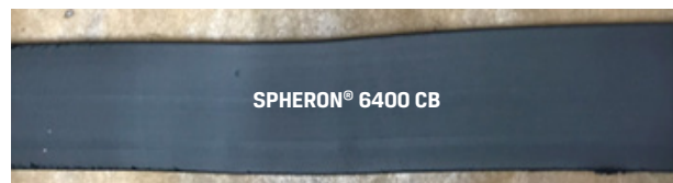
SPHERON® 6400 CB: 76 phr (24wt%), White Filler 90 phr, Density 1,300 g/liter
